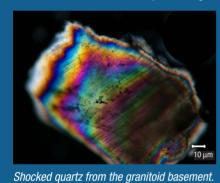
mechanism that governs impact crater formation in large impacts. The physical properties of these rocks demonstrate that the impact process reduces the density and velocity of target rocks and greatly enhances porosity.
